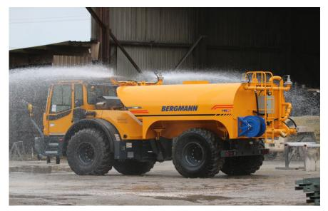
4 Tank Mounted Auxiliary Spray Heads
