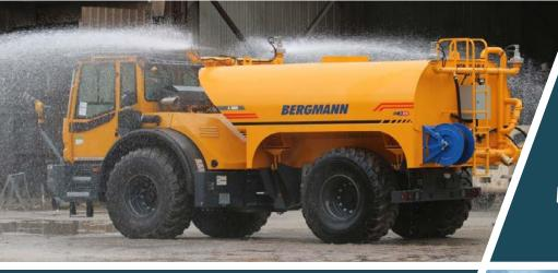
SELF-LOADING CAPABILITY AND REAR MOUNTED HOSE REEL
